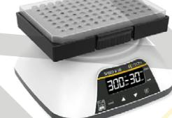
The unique plate is suitable for 96-well microplate, mixing is more convenient.
